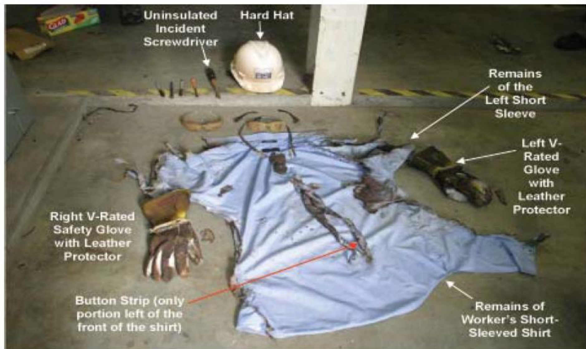
Figure 2-6. BSE-1's burned shirt and his flash-damaged PPE and tools
