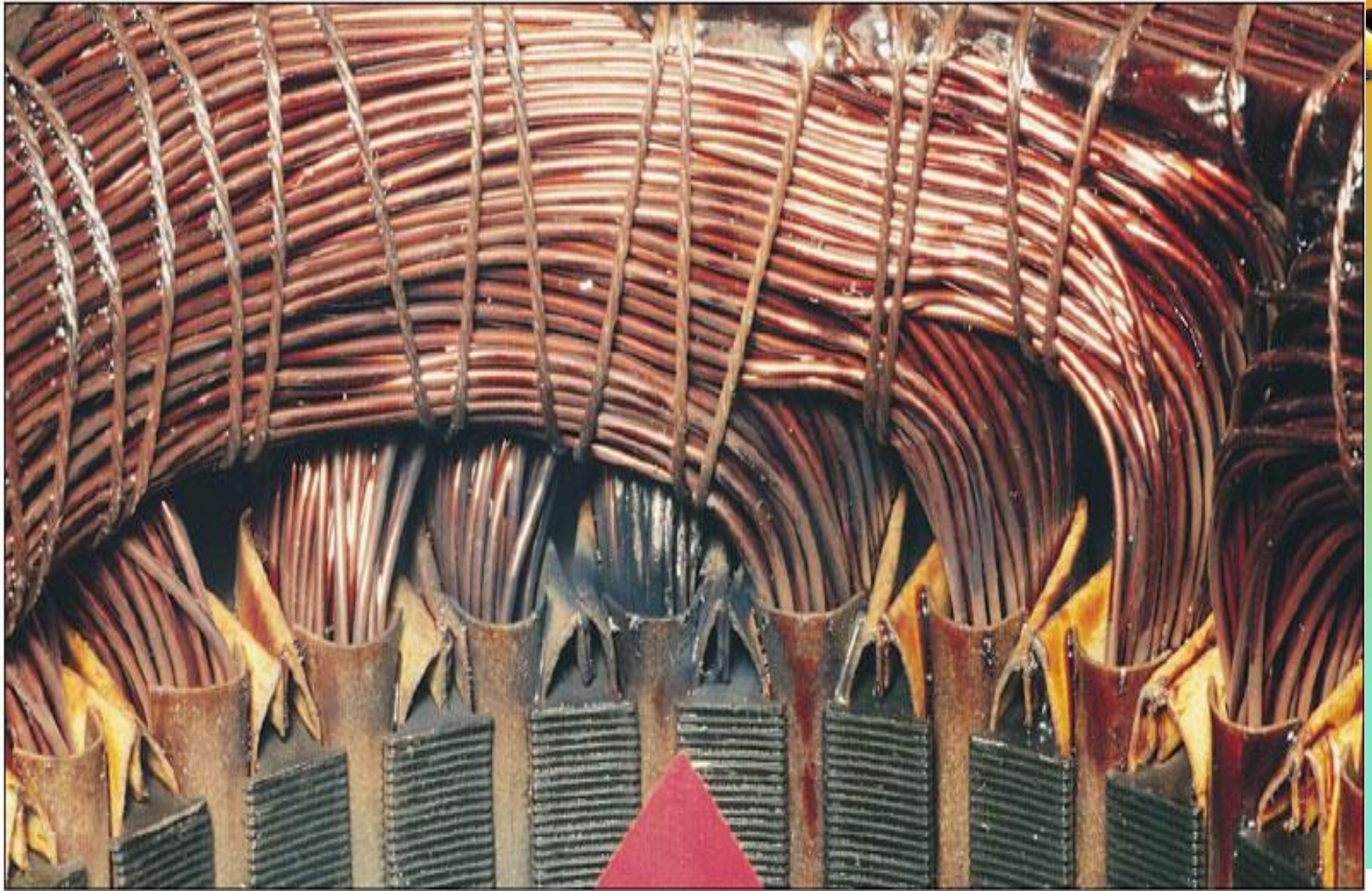
Figure 1 — If the output pulses from an IGBT-based drive travel a distance to the motor, it can reach an amplitude destructive to the motor insulation. The burned section in the photo was caused by such a reflected wave.
